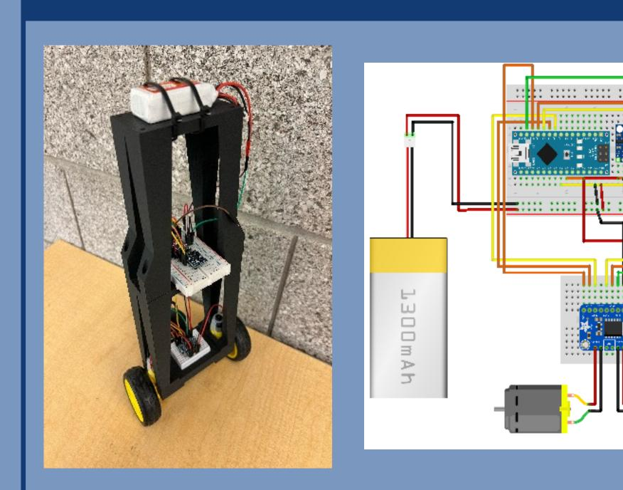
Our project revolves around a popular controls problem where a controller balances a two-wheeled vertical robot. This robot uses an Arduino Nano, MPU-6050 IMU sensor, a TB6612 Motor Driver, a 7.4V LiPo rechargeable battery, and two DC motors. We programmed the Arduino in the Arduino IDE and programmed the controller based on IMU accelerometer data to provide the feedback.
