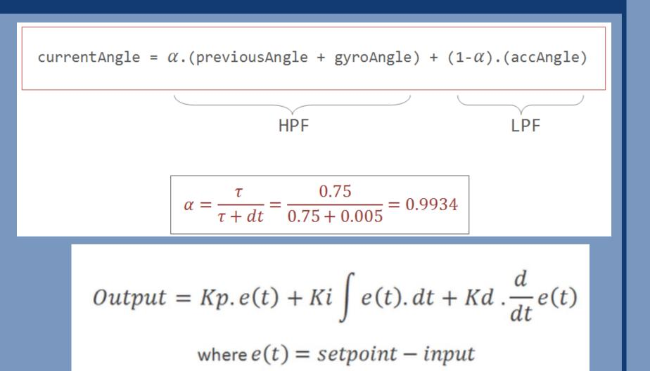
Complementary Filter Equation (top) and PID controller equation (bottom) (Source: <a href="https://www.instructables.com/Arduino-Self-Balancing-Robot-1/">https://www.instructables.com/Arduino-Self-Balancing-Robot-1/</a>)
